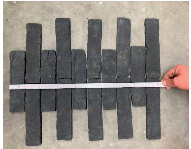
Calculating the average height of a brick slip
